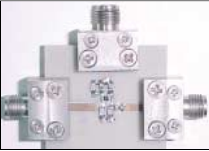
Figure 12. Photograph of the unequal Wilkinson power splitter.
